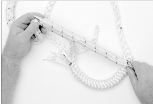
Inserting fid through cover
