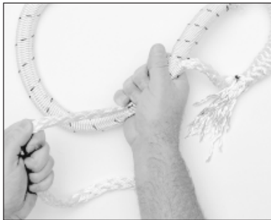
Pulling core end to tighten cross-over
