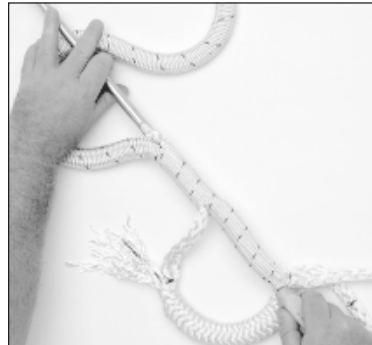
Pushing fid and core through cover
